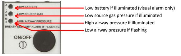
Flashing Alarm Status LEDs
